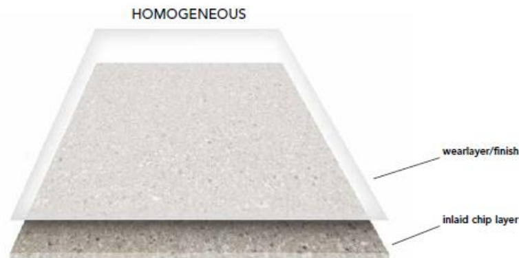
Figure 1: Diagram of homogeneous vinyl flooring cross section
